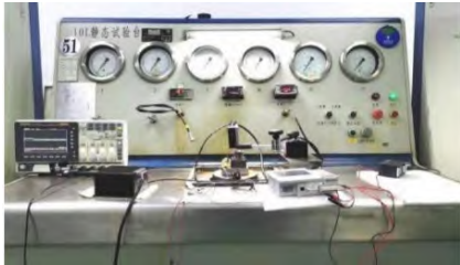
图 11 偏转板射流放大器压力特性实验系统 Fig. 11 Experimental system for pressure characteristics of deflector jet amplifier
