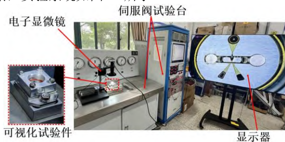
图 14. 基于显微镜的流场可视化实验实物图 Fig.14 Physical image of flow field visualization experiment based on microscope
