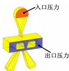
图6. 可视化试验件流场三维模型 Fig.6 Three dimensional model of the flow field for the visualization test piece
