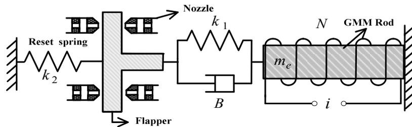
Fig.3 Sketch of GMA magnetic-mechanic coupling
