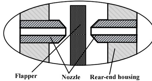
Fig. 2 Detail View of nozzle-flapper structure
