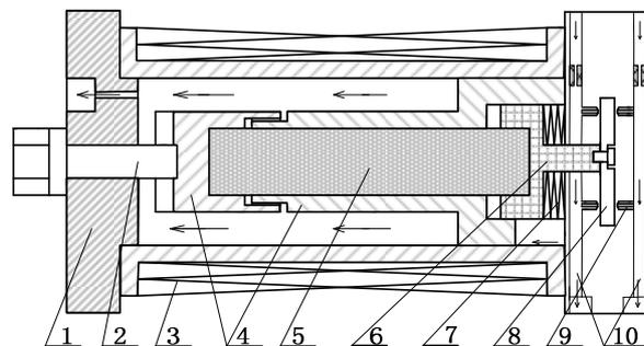
Fig. 1 Structure of four-nozzle flapper valve with GMA (1. Front-end housing, 2. Adjusting screw, 3. Driving coil, 4. Thermal compensation module, 5. GMM rod, 6. Output rod, 7. Spring, 8. Flapper, 9. Nozzle, 10. Rear-end housing)
