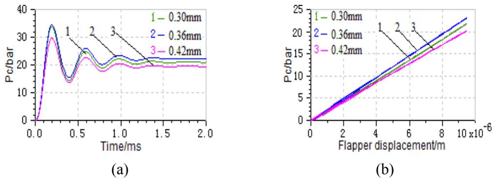
Fig. 9 Dynamic (a) and static (b) performance of control pressure with different fixed orifice
