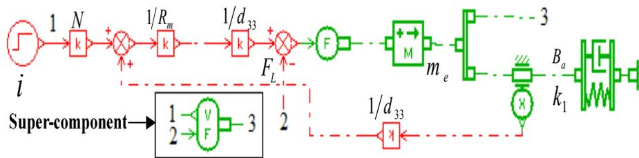
Fig. 4 AMESim model of GMM Actuator
