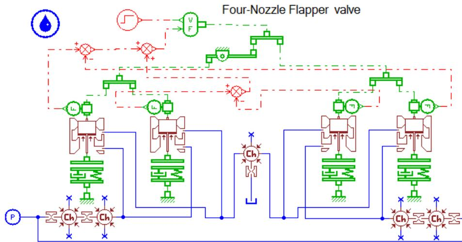
Fig. 6 Simulation model of four-nozzle flapper valve with GMA
