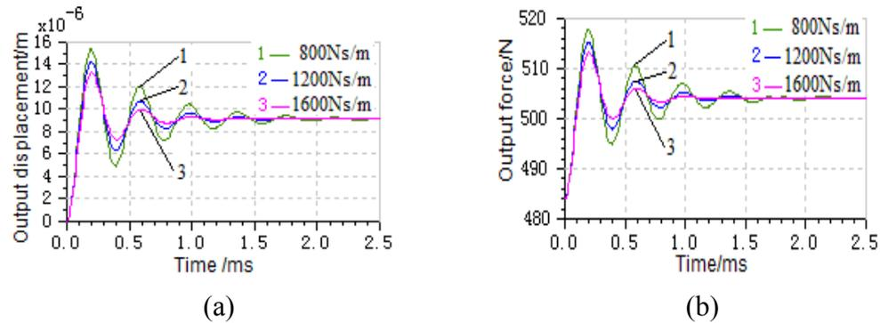
Fig.8 Step response of output displacement (a) and output force (b) with different damping coefficient
