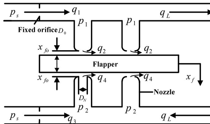
Fig. 5 Sketch of four-nozzle flapper valve
