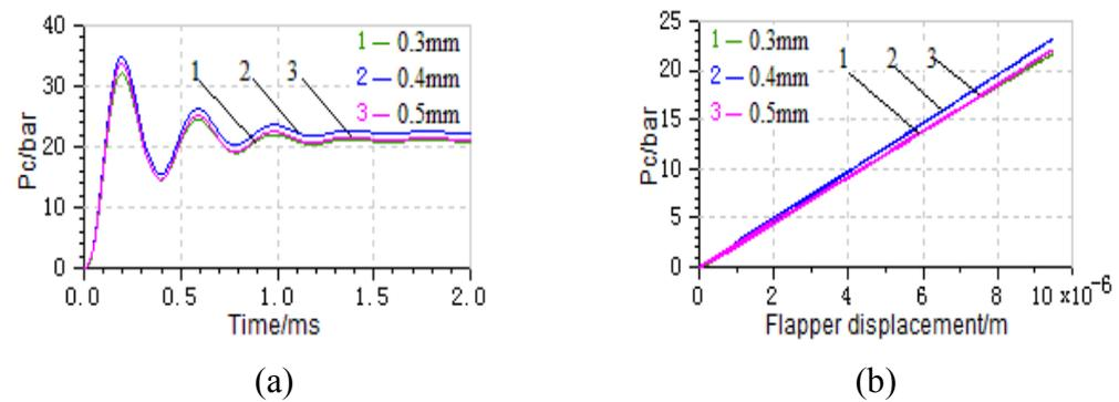
Fig. 10 Dynamic (a) and static (b) performance of control pressure with different nozzle orifice
