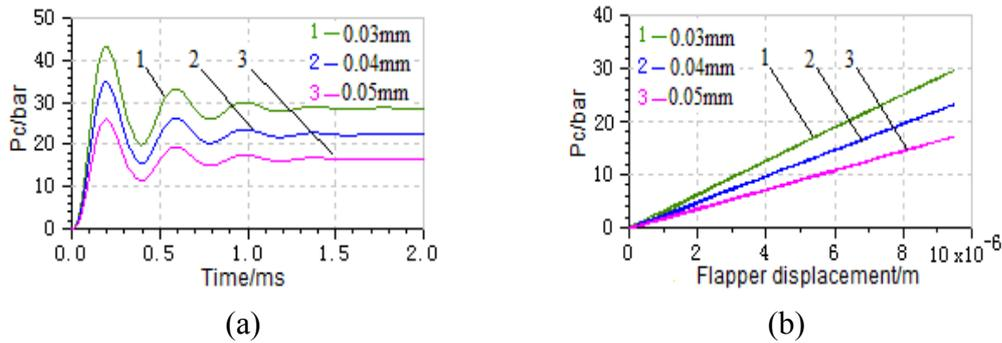
Fig. 11 Dynamic (a) and static (b) performance of control pressure with different zero clearance
