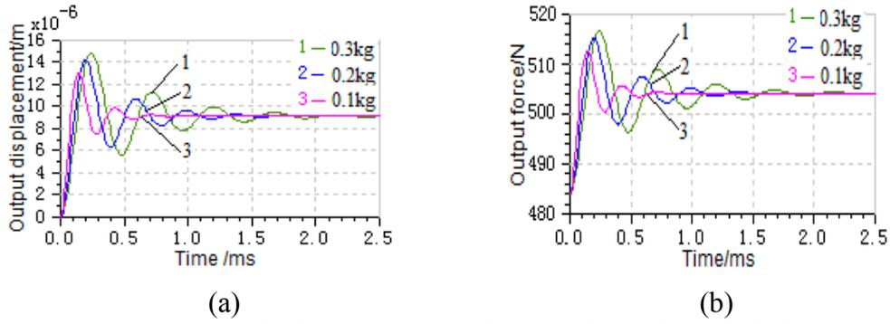
Fig.7 Step response of output displacement (a) and output force (b) with different equivalent mass
